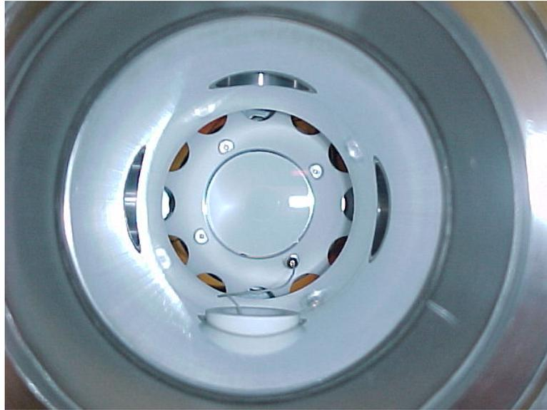
Figure 2.13: The back side of the phosphor screen that the CCD camera sees. This picture was taken before the light baffle in Fig. 2.14 was installed.
