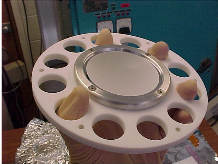
Figure 2.12: The phosphor screen in its machinable-ceramic mount. This side faces the plasma.
