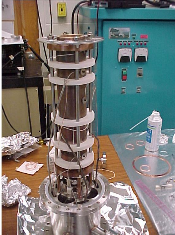
Figure 2.3: Trap electrodes and filament assembly.
