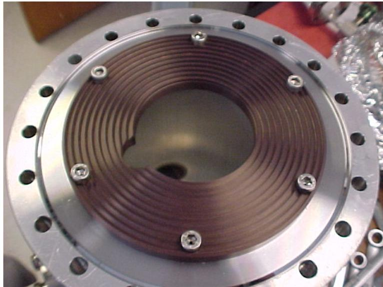
Figure 2.14: This light baffle was mounted roughly 1 inch behind the phosphor screen to block stray filament light. The inside faces of the grooves in its surface are perpendicular to its base to reduce the light reflected inwards towards the back of the phosphor screen. The offset hole in the baffle ensures a safe distance between the grounded baffle and the bias wire to the 3–5 kV phosphor screen, seen in Fig. 2.13.
